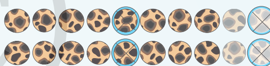
Be careful of selecting within a natural pattern. Here the biscuits at the end are under cooked but are over represented in the sample.
